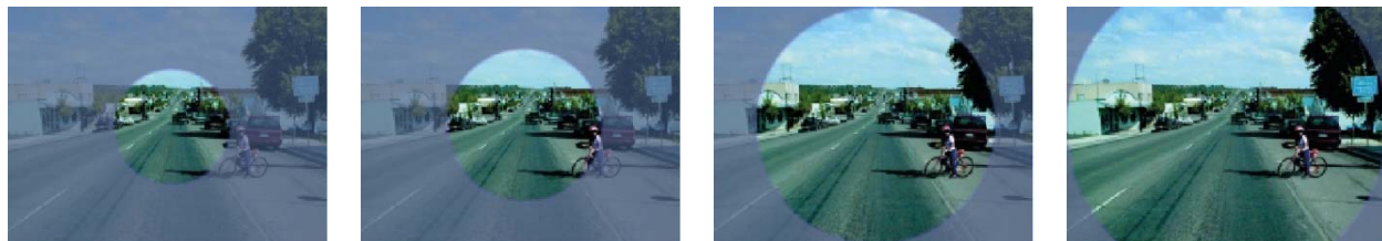
40 mph 30 mph 20 mph 15 mph Clear field of view at different speeds (from Oregon Main Street Handbook)
